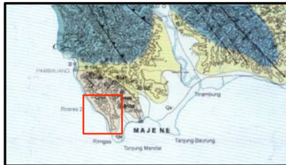
Figure 2. Geological Map of the landslide area (Qpps = Napal Pambuang, Tmm = Formation of Mandar, Tmpm = Formation of Mapi).
