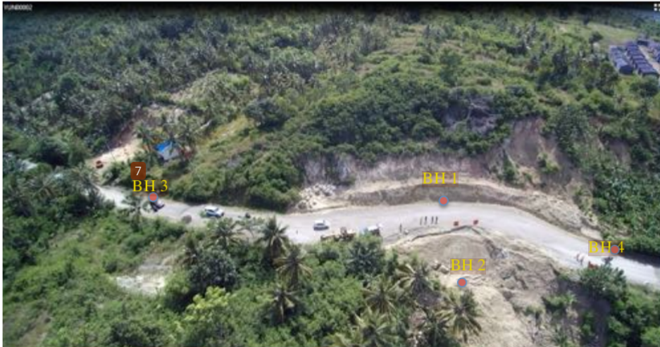
Figure 4. Layout of the boreholes location in the landslide area and the environment.
